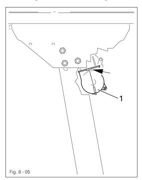
• Adjust bottom -V-belt guard **1** so that the motor pulley and V-belt run freely.
